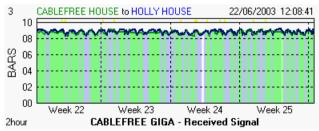
A CableFree FSO Link with ATPC enabled in identical conditions shows almost no variation in received power (RSSI). The controller automatically adjusts the transmitted power levels to ensure optimum signal received at both ends of the link.
